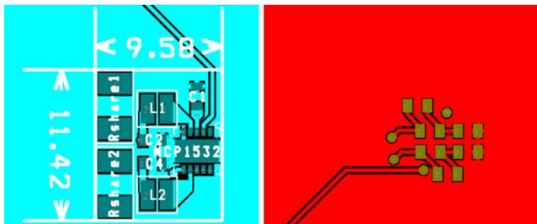
Figure 9. Load Sharing Application Top and Bottom View
